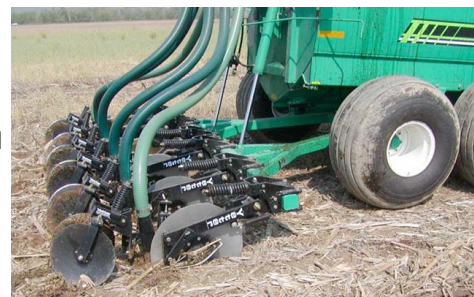
Figure 1: VA Tech's shallow, coulter-type slurry injector used in this demo project
